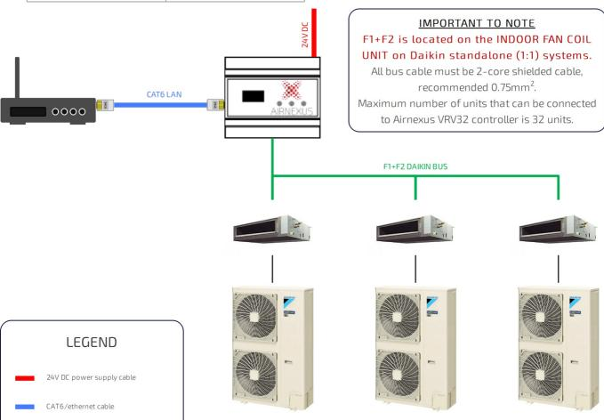
\*\* Daikin smaller domestic ranges may need an additional Daikin adapter to provide the F1+F2 connections. Please check the manufacturer's specifications for each unit type to ensure correct connections are available. \*\*
